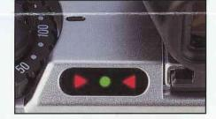
LED lamps at the rear of the camera display whether the correct exposure has been selected. The LED lamps are
